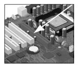
The AGP Pro 1.5V slot provides graphics performance for high-end graphics cards, combining AGP 4X bandwidth (data transfer rates as fast as 1056MB/sec) with the ability to accept high-end graphics cards drawing up that draw as much as 110W of power.
